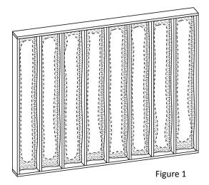
Additional lifts or passes are to be done after the initial lift or pass has had adequate time to cool down (about 15-20 minutes for two inch pass). The picture framing technique will ensure that insulation seals cracks and crevices without resulting in fold-over along the stud face or air-pockets or voids which will affect the insulations performance.
